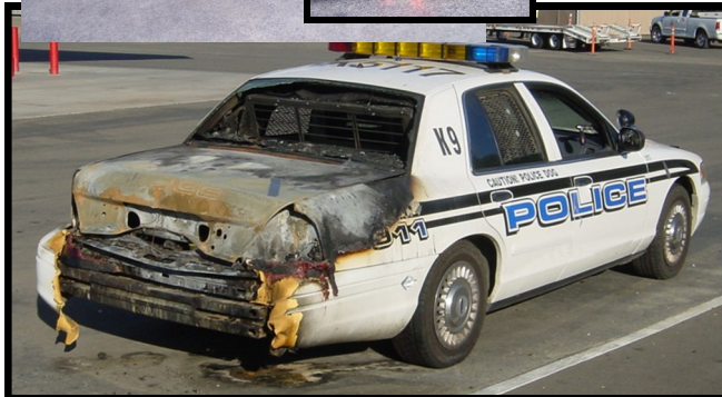
Accidental Combustion of Fusee Flares in Trunk of Police Car
